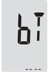
② Press the ▲ or ▼ button. The meter screen will display 'OFF', 'On', and 'PAIR' in turn. To pair your meter with your smartphone, press the ● button when 'PAIR' blinks on the screen.
